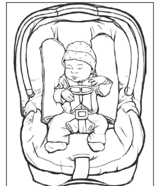
Figure 4. Car safety seat with a small cloth between the crotch strap and infant; harness chest clip positioned at the center of the chest, even with the infant's armpits; and tightly rolled receiving blankets on both sides of the infant.
